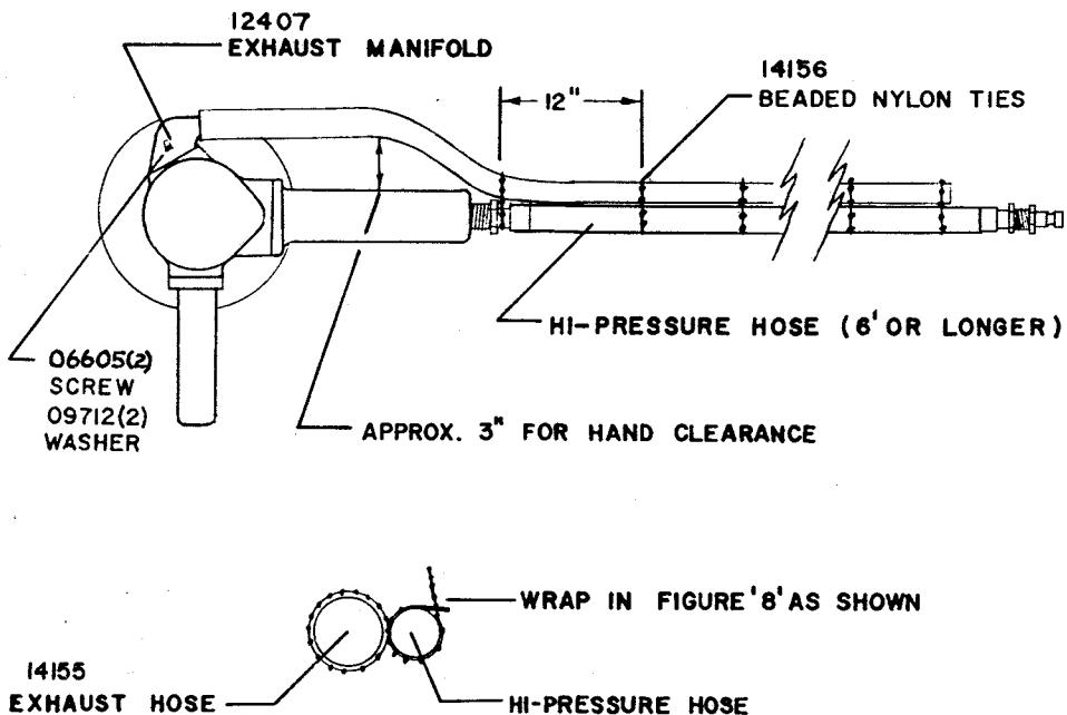
To attach a #53881 Remote Exhaust or #53882 Muffler to a V-Series Grinder, which does not have mounting holes, the holes shown below must be drilled.
